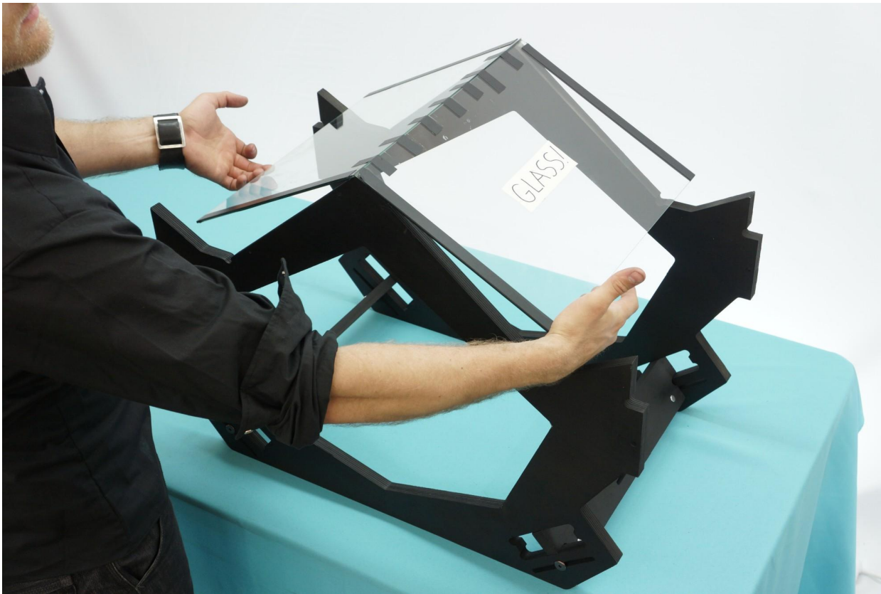
13c. Flip the Imaging Module so the pointy parts go up. Seat your glass plates on the Imaging Module. The mitered edges of the glass plates should mate cleanly into a point.
